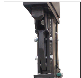
LED-work light and removable spacer block.
