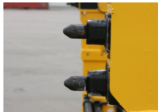
Locked twistlocks. Upper twistlocks retracts automatically 110 mm.
