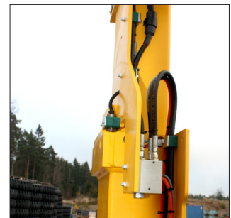
Surface-mounted hose and cable routing.
